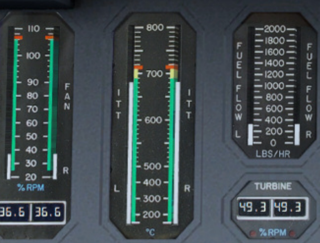
Engine Instrumentation is of the ribbon type with crisp and clear character sets and movements.
