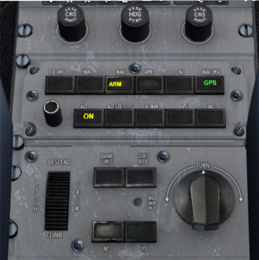
The Autopilot control unit is located in the center console as are the EFIS CRS and HDG selectors. Interesting feature of the Autopilot is the Bank limit switch and the large turn knob.
